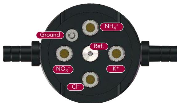
Particular attention has been paid to identify a set of sensors stable and at the same time sensitive. For this purpose, it has also been introduced a reference electrode with a particularly high performance and a high capacity of compensation of the pollutants.
